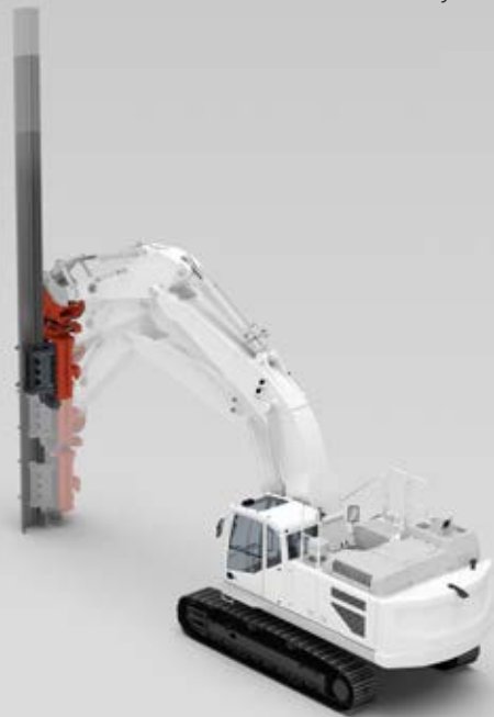
Vertical movement with a stationary excavator.
