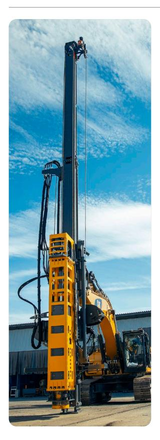
MOVAX multi-tool piling leaders provide a versatile, multitool solution for a wide range of piling requirements in a variety of site and soil conditions, and for different types of piles and piling technologies.
