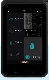
The MOVAX Control System, mControl+, links the carrier (excavator, railroader or equal) with the MOVAX piling equipment and customised solutions. The system controls the auxiliary hydraulics of the excavator which in turn is utilised to control the MOVAX piling equipment, the MOVAX multi-tool piling leaders including the tooling connected to the leader and the MOVAX column stabilisation leader.
