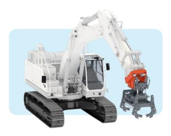
MOVAX manipulators are designed for fast, flexible and efficient handling of different kinds of masts, gantries, and poles as well as a wide range of piles. Based on the patented side grip technology, the MOVAX manipulator is designed for superior maneuverability, safety and accuracy.
