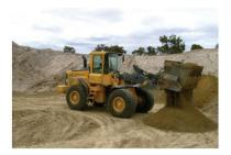
A suitable loader model is determined by the availability of hydraulic flow from the carrier unit and the type of material required to be processed.
